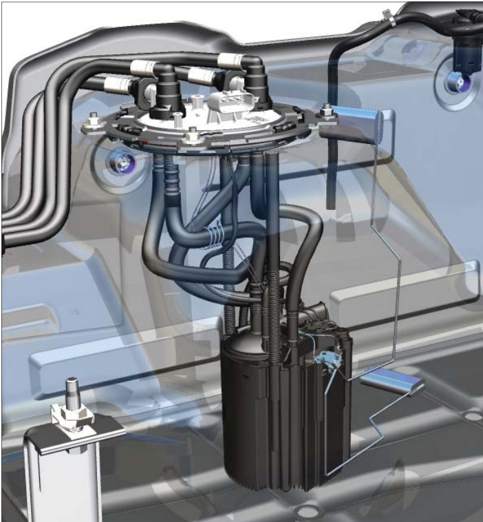
Low pressure electric fuel pump (shown with fuel tank float at full and empty)
