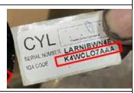
When attempting to program the incorrect IQA from the service label into the PCM an invalid values message will display: \*\*\* THE VALUES DISPLAYED IN 'RED' ARE INVALID \*\*\*
